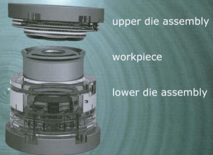
CCIF forging tooling and workpiece
