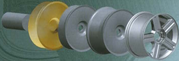
Production flow from billet to finished SUV wheel
